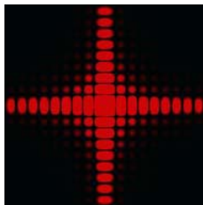
Figure 9.6 The diffraction pattern when light passes through a small square hole in a plate.
